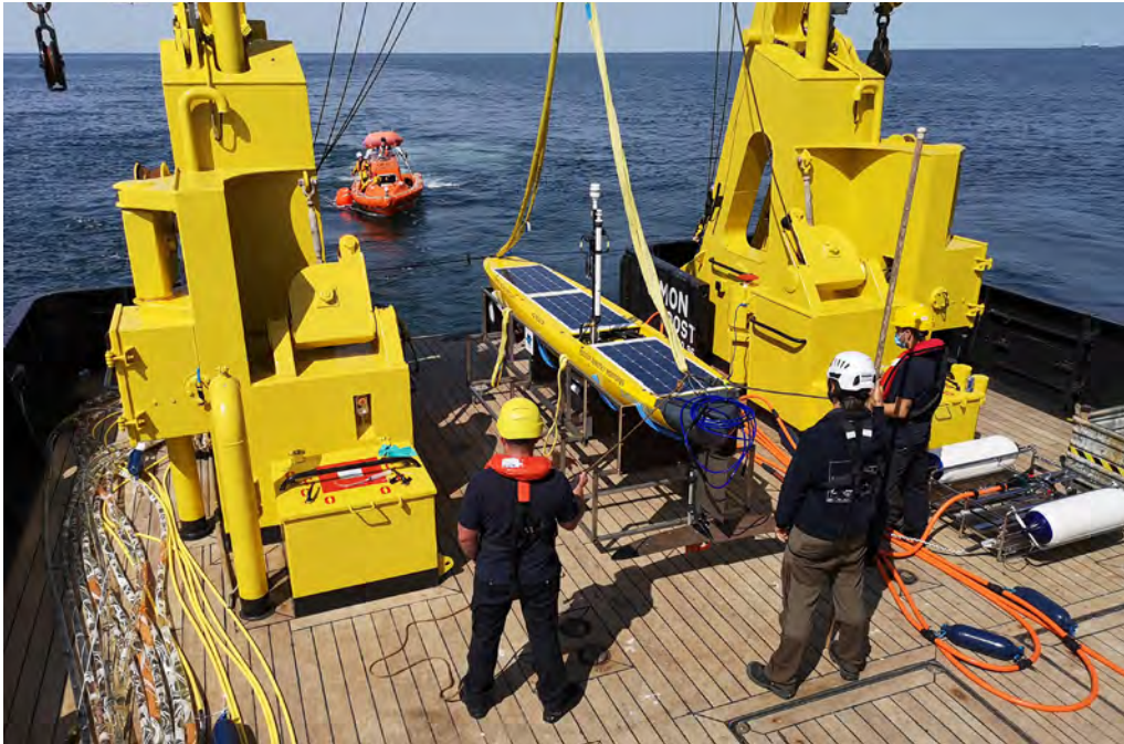
The uncrewed surface vehicle (USV) Adhemar on board RV Simon Stevin in June 2020. © VLIZ
