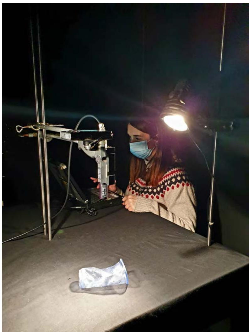
Researchers from VLIZ collect light spectra of plastic litter in a VITO laboratory for the PLUXIN research project. Within the context of the PLUXIN research project, VLIZ, VITO, Ghent University, the University of Antwerp and KU Leuven joined forces with Blue Cluster and 13 companies to monitor plastic pollution in several Flemish ports and rivers by means of innovative methods. © VLIZ
